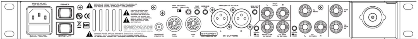
1. **AC MAINS INPUT** – Connect to a grounded outlet in accordance with the voltage and frequency specified on the rear panel of your amplifier.
