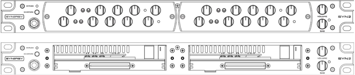
**REPLACING MODULES:** When inserting or removing modules, simply turn both thumbscrews to the left until they fall loose. Do not remove the screw completely. Remove the module by pulling out on the thumbscrews. Slide in a new module, and push in on the center knobs until flush with the front panel. Tighten the thumbscrews, by turning to the right until snug. The thumbscrews must be snug for proper module grounding. You don't need to "crank" them down but do not leave them loose.
