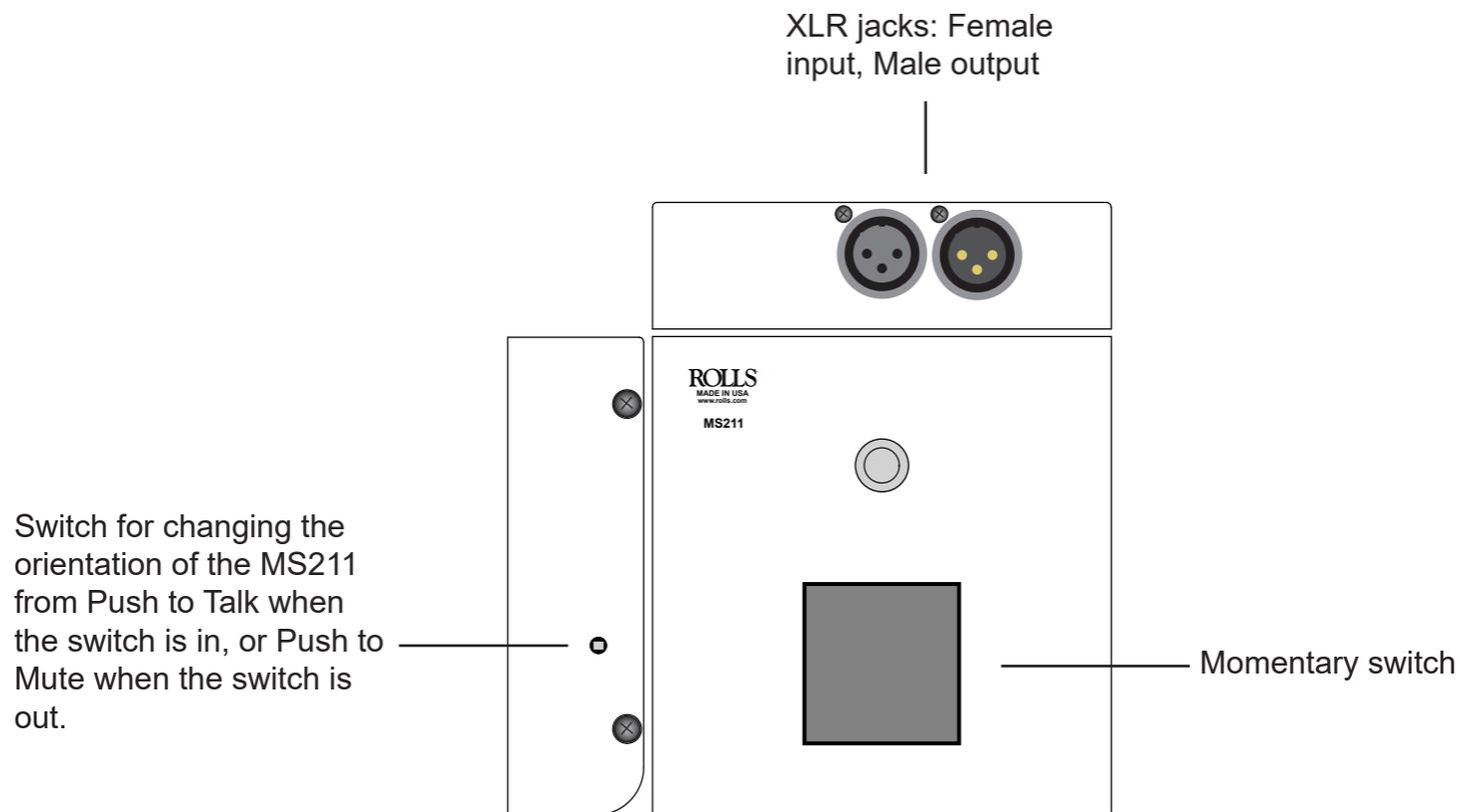
The MS211 rear panel has two screw holes for convenient mounting.
