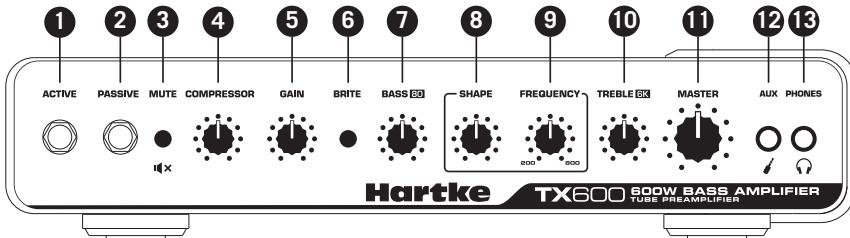
1. **PASSIVE Input jack** - If your bass guitar has passive circuitry, connect it here. This standard, 1/4" unbalanced jack provides a high impedance ( $100\text{ k}\Omega$ ) input sensitivity of 20 mV.
