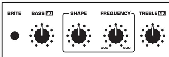
The SHAPE and FREQUENCY knobs apply an adjustable notch (scoop) filter to the specified frequency area, so that you can customize the effect of the EQ curve that best complements your particular bass instrument. As the SHAPE knob is rotated clockwise the depth of the notch increases. Moving the FREQUENCY control clockwise causes the notch filter to be applied to higher frequencies, while moving the knob counterclockwise causes it to be applied to lower frequencies.
