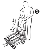
3. To lower handle, press the release lever and push down and foward to release handle from its locked position
