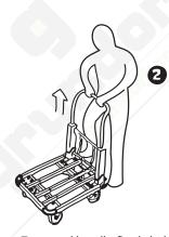
2. To extend handle, firmly hold the platform and pull the handle up until it is locked into position.
