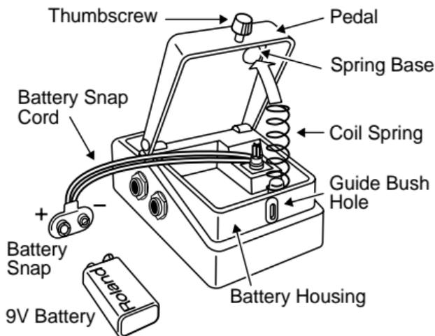
1. Loosen the thumbscrew at the front of the pedal, then lift the pedal upwards to open the unit.
