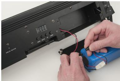
5. Carefully disconnect the battery cables.
