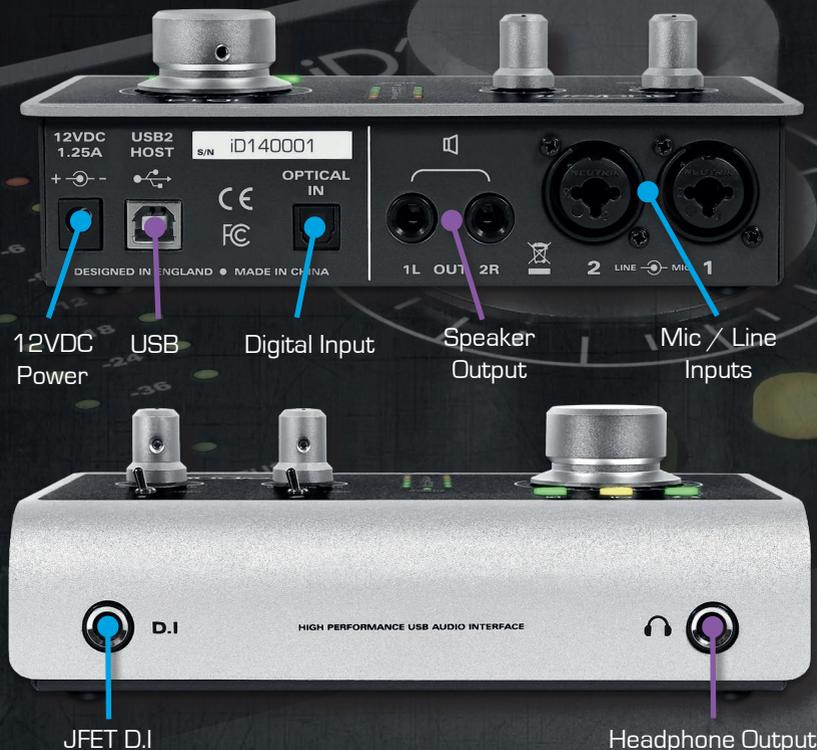
iD14 features flexible monitor and volume control using the encoder and the encoder select buttons which can help improve your workflow.
